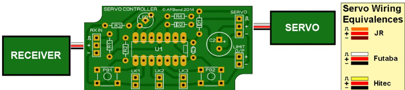
If a sound trigger is to be used, simply plug a male two pin lead onto the "limit o/p" header and connect the other end to the appropriate trigger input you wish to use. Be sure to mate the "-" contact of the "limit o/p" header with the 0v contact on the sound trigger unit. Detailed instructions about using the latter are beyond the scope of this document and you should consult the sound unit manufacturer's documentation.
