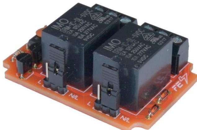
To gain access to the jumper links, the lid of the unit requires to be opened by removing the 4 screws. *When replacing the lid, take care not to over-tighten the screws lest you strip the threads in the plastic case.*
