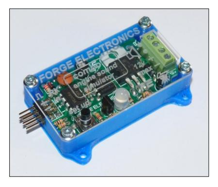
This engine sound simulator is principally intended for radio controlled model boats but may also find application in trucks, tanks, cars, rock-crawlers and even aircraft.
