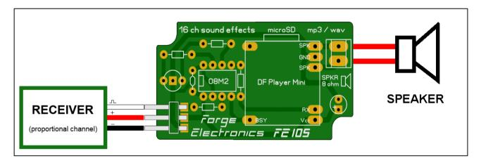
If the unit is plugged in the wrong way round to the receiver, no damage will result but the unit will give a continuous low frequency rhythmic pulsing sound from the speaker, accompanied by a flicker of the LED
