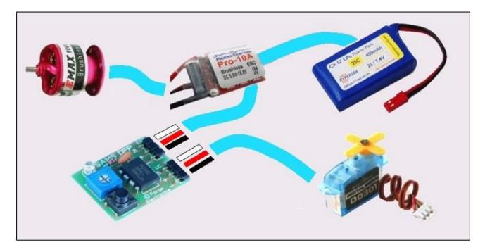
The signal lead from the ESC, usually coloured white/red/black, connects to the top three pin header on the timer as shown in the image above and the U/C servo to the lower three pin header. Note the orientation of white/red/black leads.
