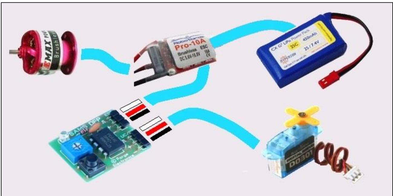
The signal lead from the ESC, usually coloured white/red/black, connects to the top three pin header on the timer as shown in the image below and the D/T servo to the lower three pin header. Note the orientation of white/red/black leads. The remote push button and/or remote LED (if used) are connected to the two pin headers as shown. This information is also repeated on the label of the timer (shown here unpackaged for clarity).
