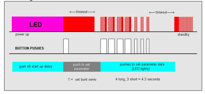
When modifying the bunt servo duration, if the user enters a duration which equals or exceeds the current DT period, then when the timer reverts to standby mode to prevent the user operating with this dangerous condition, the timer is inhibited and enters an endless loop with the LED showing permanent MAGENTA. Power must be cycled and the bunt servo or DT period altered to safe non-overlapping values.
