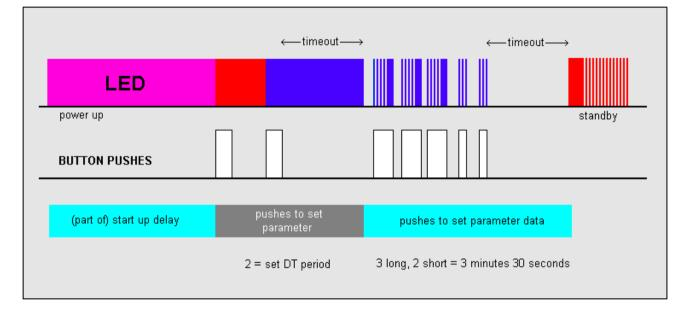
When modifying the DT period, if the user enters a duration which equals or is less than the bunt servo period, then when the timer reverts to standby mode to prevent the user operating with this dangerous condition, the timer is inhibited and enters and endless loop with the LED showing permanent MAGENTA. Power must be cycled and the bunt servo or DT period altered to safe non-overlapping values.
