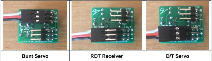
The silk screening on the PCB identifies the ESC connector (used for bunt servo) and the polarity of its connections. Note the silk screened 'RDT' and 'D/T' legends are aligned to the connector's soldered pins so users may trace back to which row of pins to plug into if this document is not to hand.
