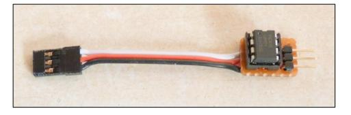
The module is available as an accessory and is supplied with a standard Futaba receiver lead.
