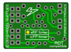
This PCB is also used for an IC Free Flight Timer version, which of course has different firmware, so to distinguish between the two variants, the PCB underside is marked with a yellow paint blob against the appropriate legend.
