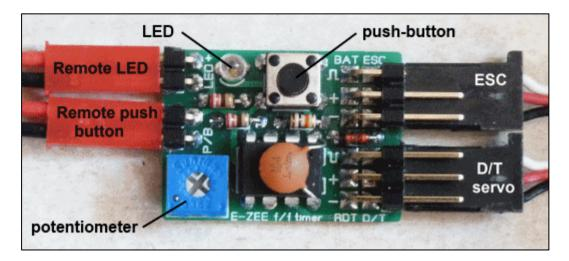
The image above shows the various leads connected to the timer in close up.
