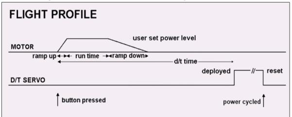
When modifying ANY of the duration settings, if the user enters a duration which causes the DT period to be less than or equal to the total running time of the motor (ie ramp up + motor run + ramp down) this setting is not accepted and the LED gives three rapid blinks repeated at one second intervals to warn the user of this dangerous conflict. Pressing the button returns the user to standby mode with the previous (safe) duration value intact.
