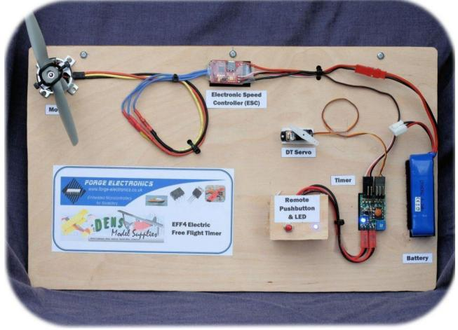
This image shows the system components, note that power does not flow through the timer. The timer is fed from BEC (Battery Eliminator Circuit) provided by the ESC and in turn sends signals to the ESC and the DT servo. <u>So the timer can be used with any size of motor/ESC/battery combination subject to the following warning</u>
