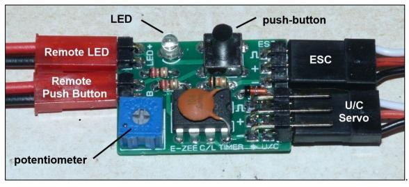
The previous image above shows the various leads connected to the timer in close up.
