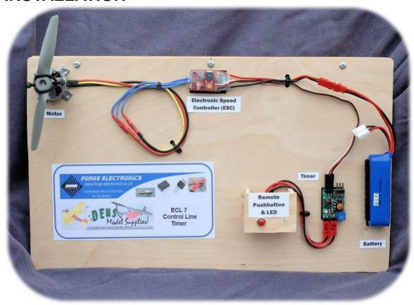
This image shows the system components, note that power does not flow through the timer. The timer is fed from BEC (Battery Eliminator Circuit) provided by the ESC and in turn sends signals to the ESC.
