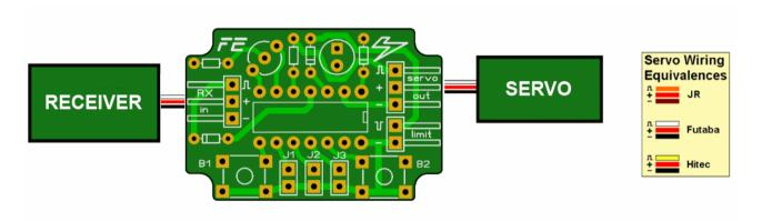
If a sound trigger is to be used, simply plug a male two pin lead onto the "limit" header and connect the other end to the appropriate trigger input you wish to use. Be sure to mate the "-" contact of the "limit o/p" header with the 0v contact on the sound trigger unit. Detailed instructions about using the latter are beyond the scope of this document and you should consult the sound unit manufacturer's documentation.
